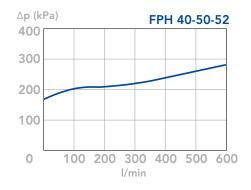
CLEAN FILTER ELEMENT PRESSURE DROP WITH C+ AND M+ MEDIA (depending both on the internal diameter of the element and on the filter media)
