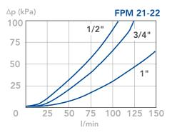
CLEAN FILTER ELEMENT PRESSURE DROP WITH F+ AND C+MEDIA (depending both on the internal diameter of the element and on the filter media)
